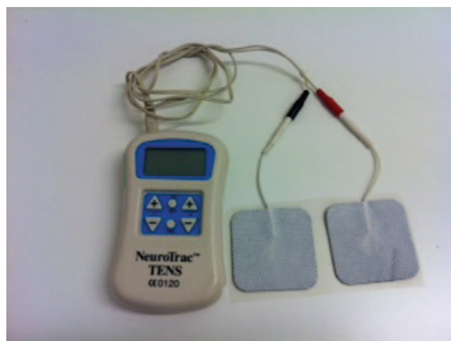
FIGURE 1. Neurotrac TENS machine (approximately 10 cm × 6 cm × 2 cm). TENS = transcutaneous electrical nerve stimulation.
